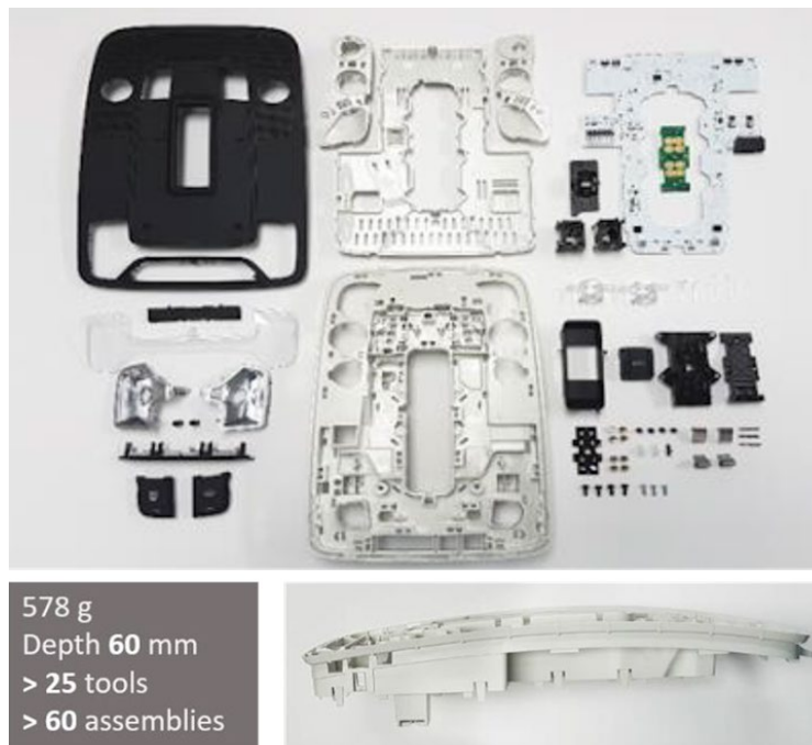
Figure 8: Conventional electronic elements for manual mounting and assembly on a real curved part.
